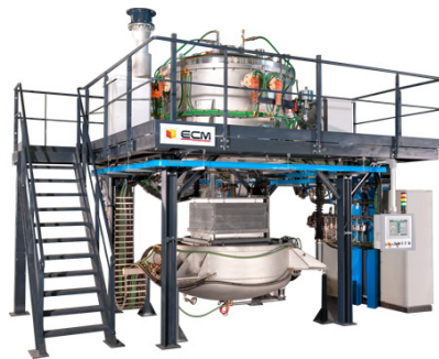
Machine ECM Greentech. Lingot de Silicium monocristalin
